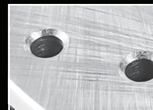
BEVELED DRILL HOLES
